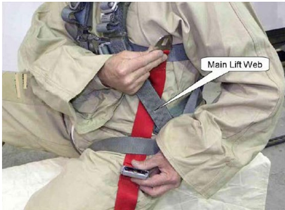
FIGURE 5. PASS TETHER LOOP UNDER MAIN LIFT WEB
