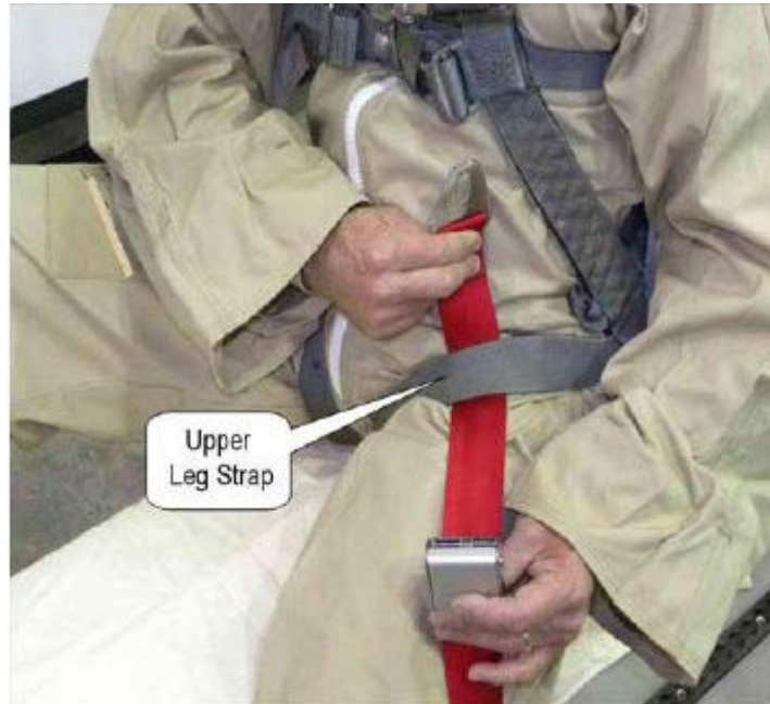
FIGURE 5. PASS TETHER LOOP UNDER MAIN LIFT WEB
