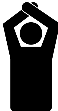
Canopy Down (CD) Down Landing (DN)
